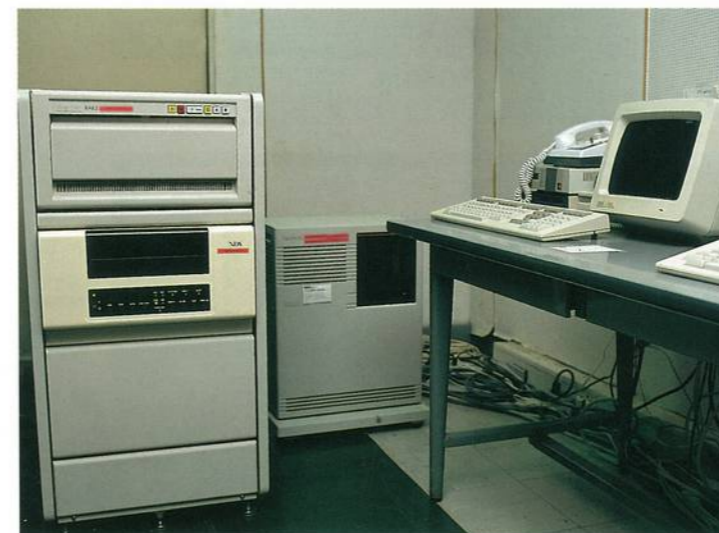
▲データ処理・交換・蓄積用コンピュータ(マイクロVAX) Micro-Vax Computer System for Data Process- ing, Exchange, and Storage
