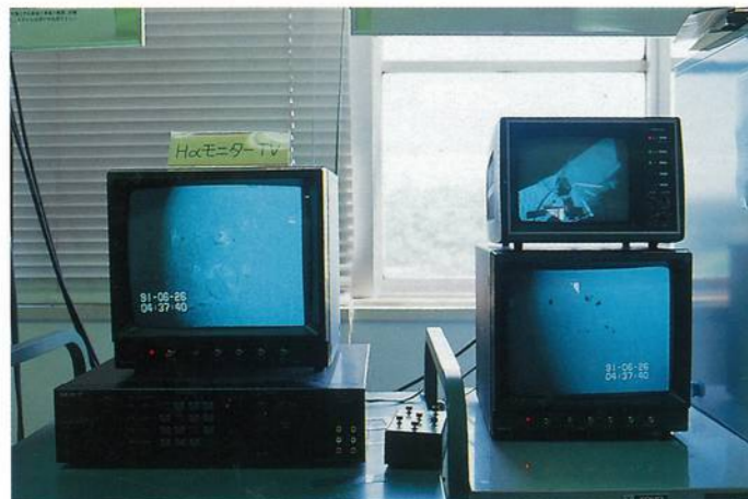
▲太陽像モニター装置(左; H \alpha 線、右; 白色光) TV Monitors of H-alpha (left) and White Light (right) Solar Images
