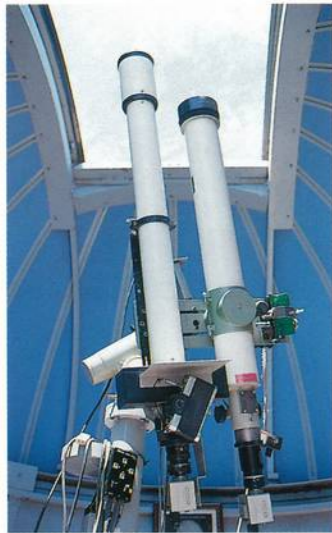
▲太陽の白色光像とH \alpha 線像観測用望遠鏡 Telescopes for White Light and H-alpha Solar Images
