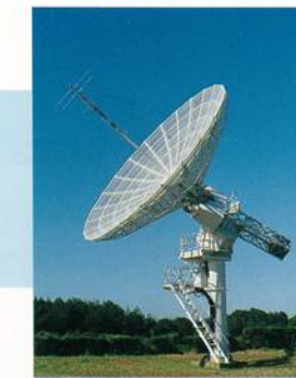
HiRAS-2 (70-500MHz) 10m赤道儀式パラボラアンテナ 10-m parabolic dish antenna with an equatorial mount
