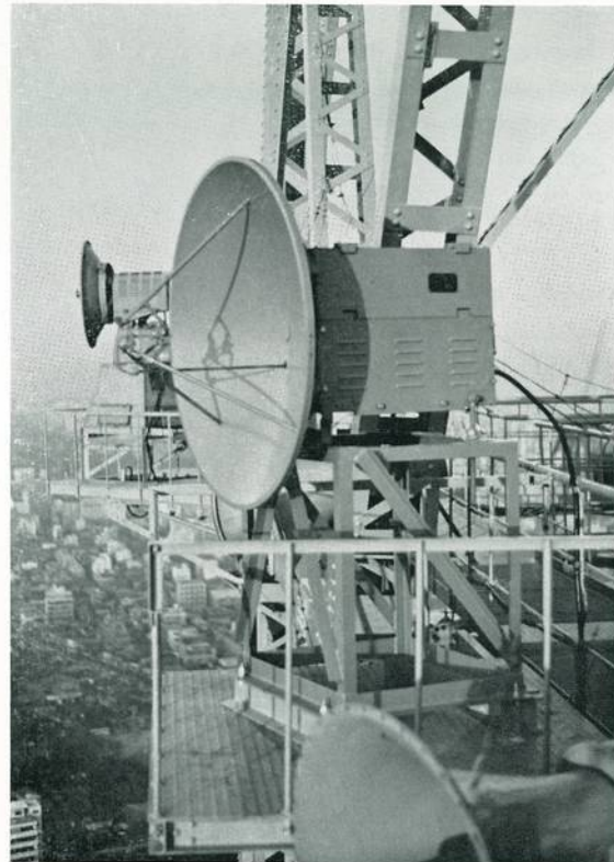
Terminal Station on the Tokyo Tower, Experiments of Propagational Characters of 8.6mm Wave on the 24 km Path.
