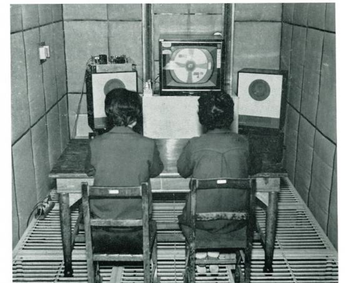
Assessment Room where Qualities of Television or Audio Signals are evaluated. It is a Room Darkenable, Sound-Proof, and Air-conditioned.
