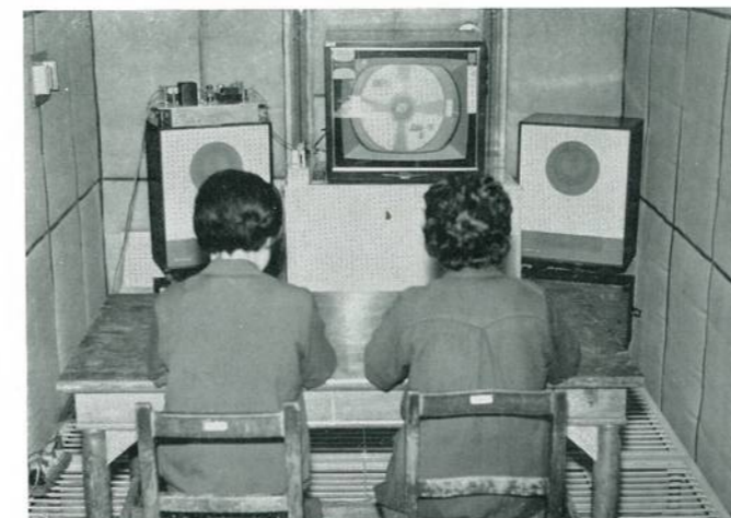
Assessment Room where qualities of television or radio signals are evaluated. It is sound proofed and air-conditioned.
