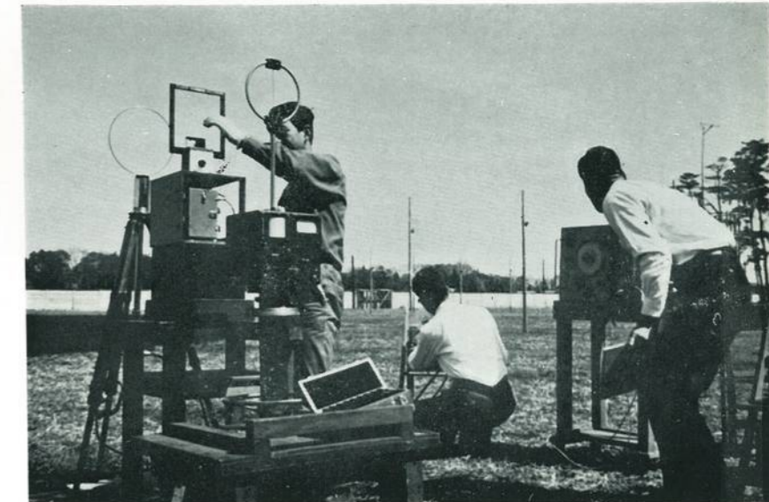
Testing of Field Strength Meter
