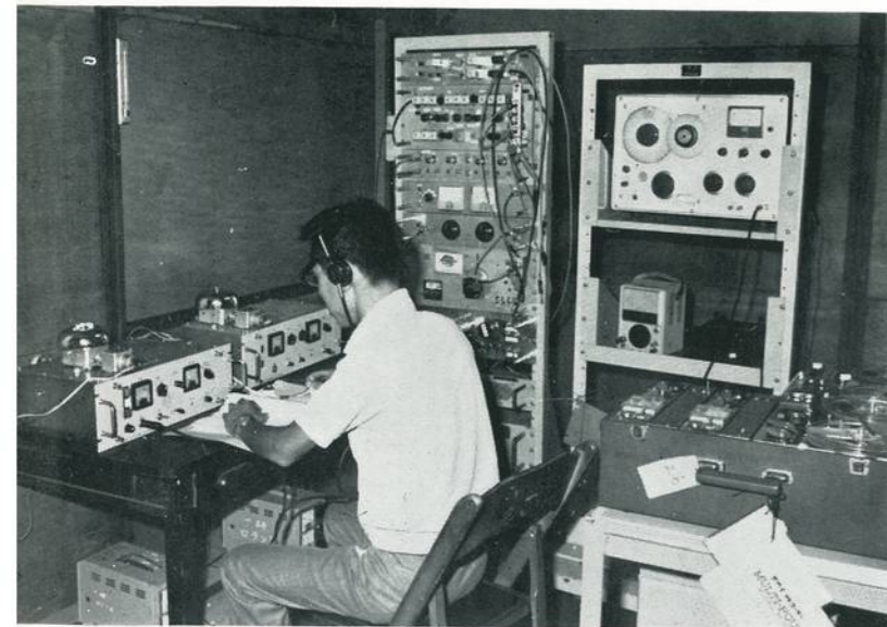
Testing of Automatic Alarm Signal Receiver
