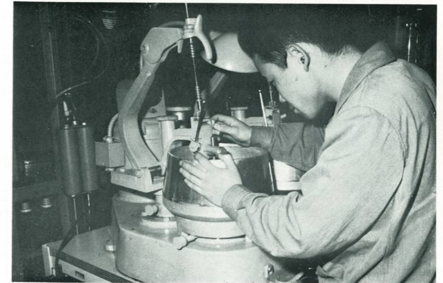
Polisher for Crystal Resonator
