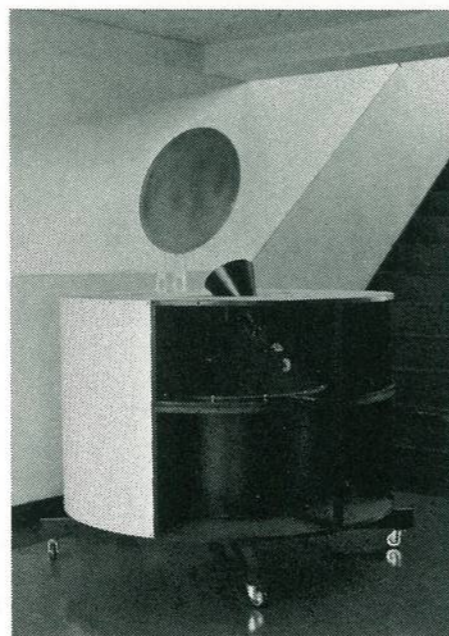
A mechanical despin antenna of corrugated horn-offset parabolic antenna type
