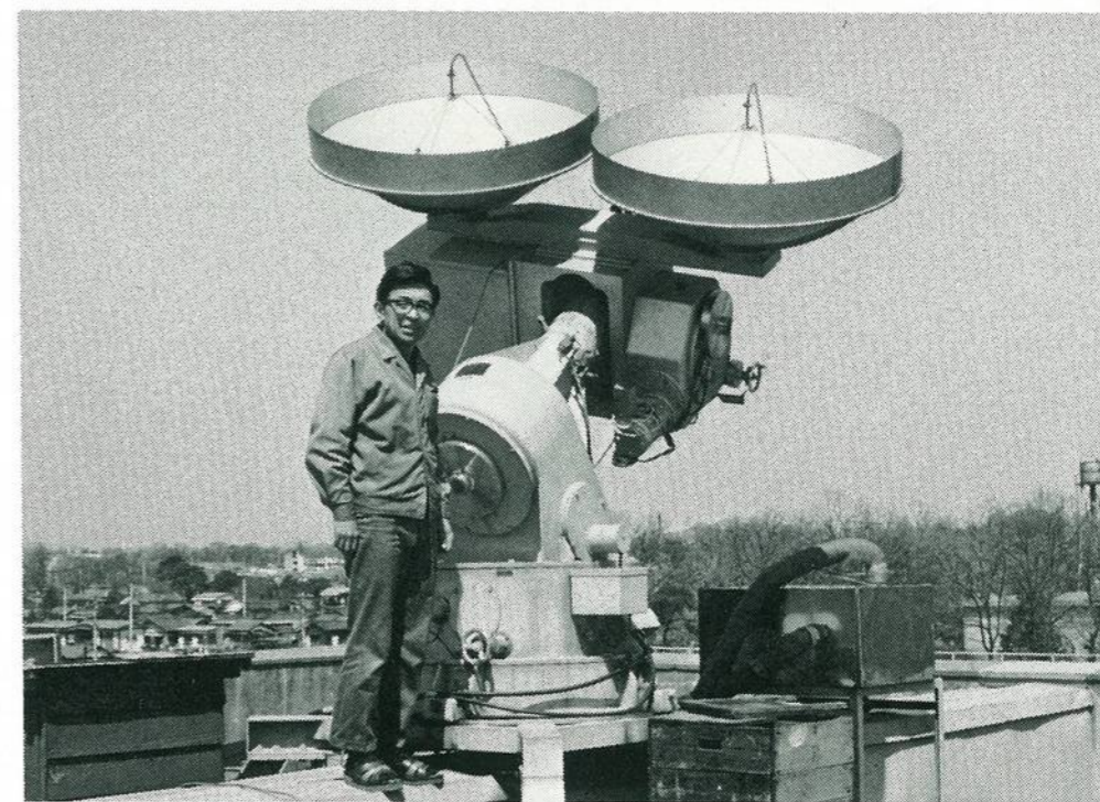
A sun-tracker for observation of mm wave propagation characteristics
