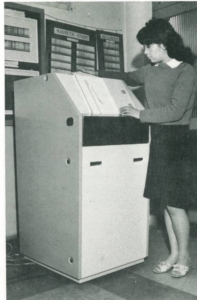
Ionofax, direct recording system for ionogram using by optical fiber tube
