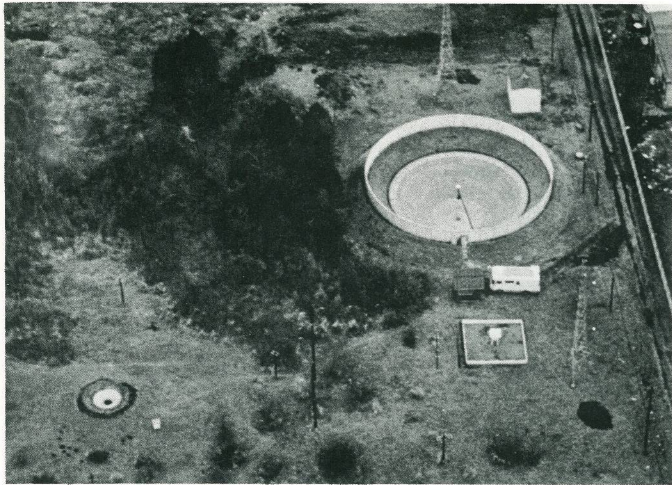
A 16-meter concrete paraboloidal dish and a 3-meter metal dish for acoustic sounding.
