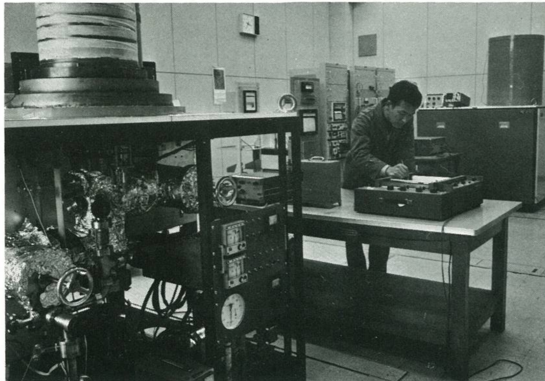
Hydrogen maser type atomic standard
