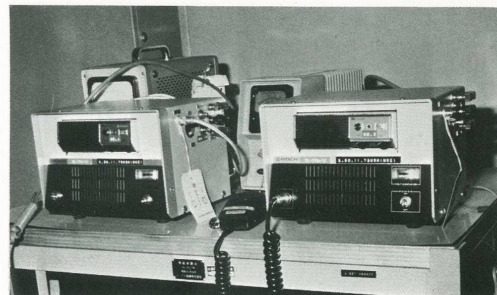
An equipment with usual band transmitter and narrower band receiver (left), an equipment with narrower band receiver and usual band transmitter (right) FM equipments with bandwidths changeable from usual to narrower ones, such equipments being used as a simplex operation in the 150 MHz band
