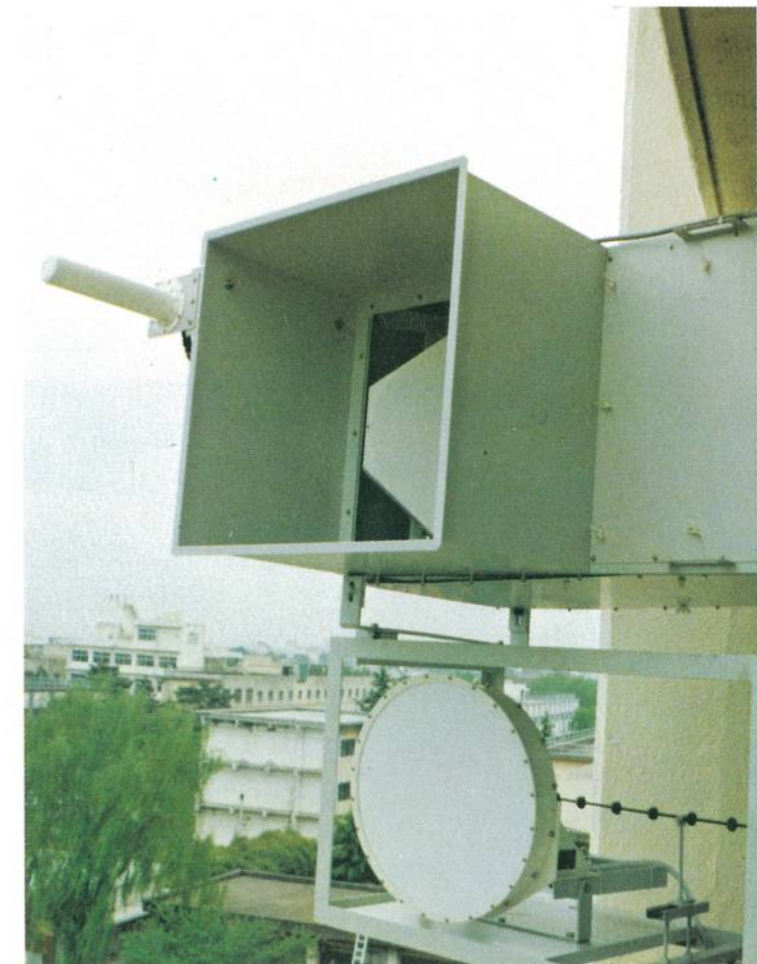
Receiving antenna system (top to bottom) 1.7 GHz helical, 11.5/34.5 GHz offset paraboloidal and 81.8 GHz Cassegrain antennas
