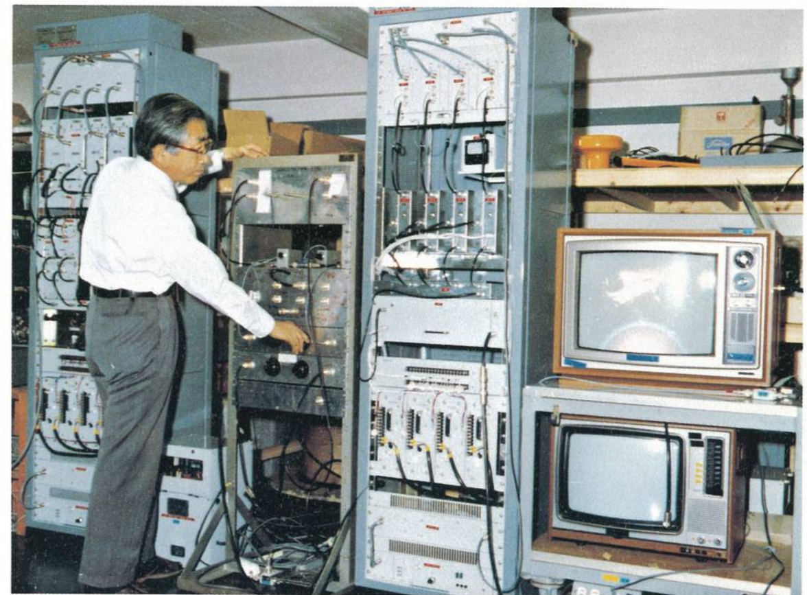
53FG small power TV translator (10W & 3W trial set)
