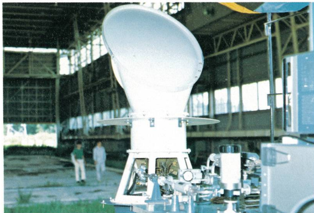
Experiment of millimeter wave attenuation due to rainfall by an FM-CW radar
